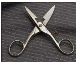
*Buttonhole Scissors – these have a small screw that can be turned to adjust the blade, creating cuts of certain lengths. The notch in the blade allows buttonholes to be made without cutting the edge of the fabric.*
